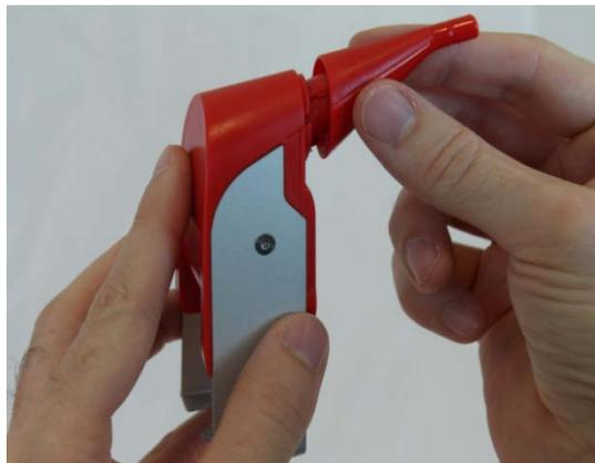
Figure 14: Placing the mouthpiece
