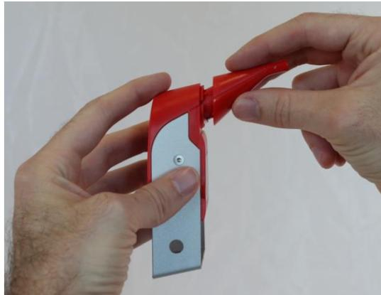
**Figure 10: Removing the mouthpiece**
