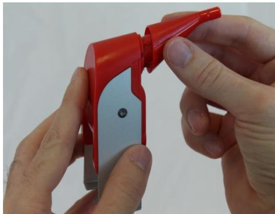
Figure 14: Placing the mouthpiece
